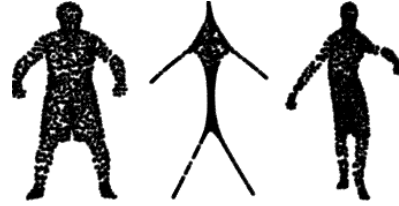
Fig. 3. The effect of joint filters is easily visualized for the case of a dynamic mesh of a dancer. By filtering the original mesh (left) using a joint low-pass separable filter one approximates the time-varying skeleton of the dancer (center). Using a non-separable wave filter, the fluidity of the dancer’s motion is emphasized (right).
